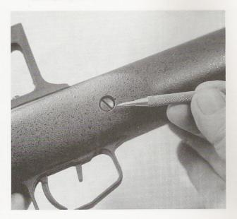
2 Remove the screw at the rear, between the port cover and the buttplate.
