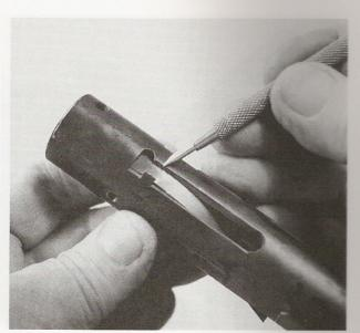
Re-hook the trigger rod and grip safety rod to their bars in the firing system before the system housing is swung back upward into place. The proper arrangement is shown.
