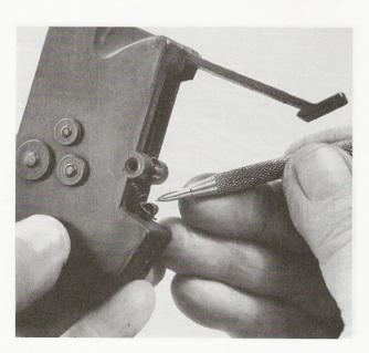
23. Unhook the grip safety spring from its post at the bottom of the housing.
