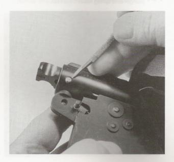
**14.** Pull the firing system housing downward at the rear, as shown.
